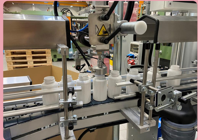
Pic.2. Leak test of the jars with compressed air.
