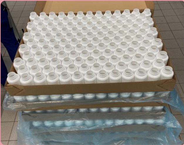
Pic. 5&6 Present packaging system for JBJ PET jars
